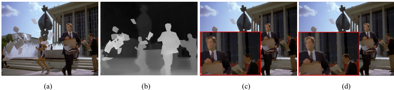
Figure 1: Image abstraction comparison between anisotropic kuwahara filtering and depth-based anisotropic kuwahara filtering: (a) original image; (b) depth map; (c) image abstraction result using anisotropic kuwahara filtering; (d) image abstraction result using depth-based anisotropic kuwahara filtering.
